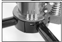
4. Lightly tighten all three bolts that hold the ram onto the leg base.
