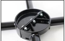
3. Now that the 3 bolts underneath have been lightly fastened, flip the legs over and place the Transmission Lifter ram onto the leg base & match up with the bolt holes.
